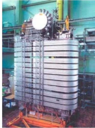
**Fig. 4.** The mechanically reinforced EURATOM LCT coil for its re-installation into TOSKA.
