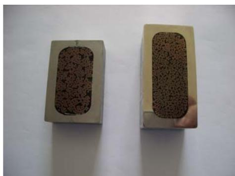
**Fig 8.** The rectangular NET conductors (CS and TF)
