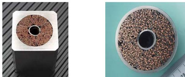
**Fig.10.** The ITER conductors (CS on left, TF on right side)
