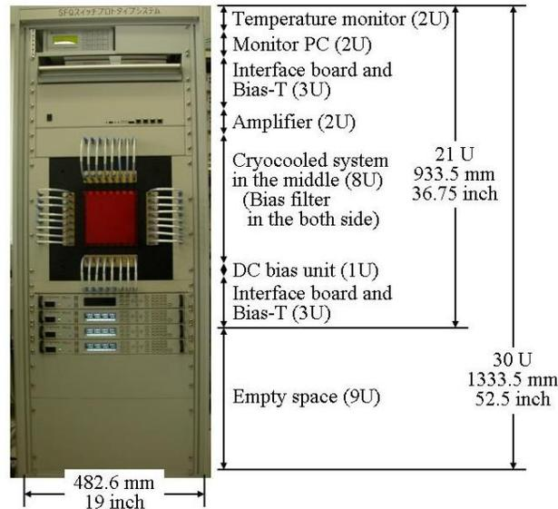
Fig. 2. The cryocooled network switch installed in a 19 inch rack (photo – courtesy of Y. Kameda).
