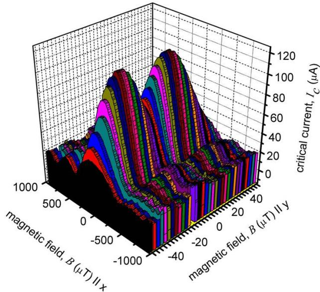
**Fig. 2.** Experimentally measured dependence of the critical current of a  $0-\pi$  sample at  $T=4.2$  K. For  $B_y=0$ , the critical current shows a regular Fraunhofer pattern. For  $B_x=0$ , a minimum around  $B_y \sim 0$  is visible which is a characteristic feature of  $0-\pi$  JJs.
