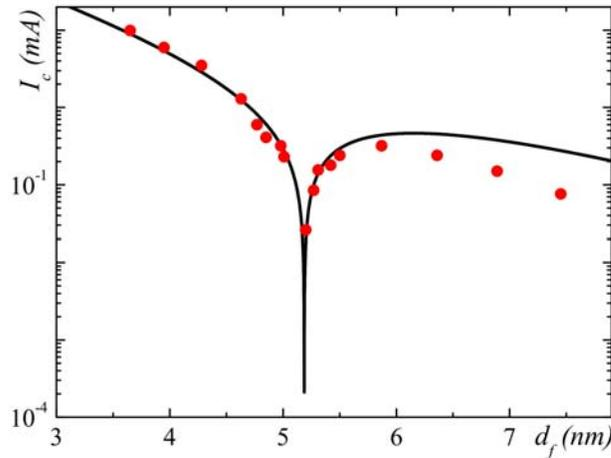
**Fig. 1.** Fit to the experimental data for the critical current  $I_c$  as function of F-layer thickness  $d_f$  in a Nb/ $\text{Al}_2\text{O}_3$ / $\text{Ni}_{0.6}\text{Cu}_{0.4}$ /Nb junction. The fitting parameters are the exchange field and the spin-flip scattering time in the ferromagnet.
