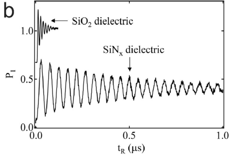
**Fig. 1.** (a) Micrograph of Josephson phase qubit circuit. (b) Rabi oscillations for phase qubit circuits incorporating PECVD-grown SiO<sub>2</sub> and SiN<sub>x</sub> wiring dielectrics. The factor 20 improvement in loss tangent for the SiN<sub>x</sub> compared to the SiO<sub>2</sub> yields a factor 20 enhancement in qubit energy relaxation time. Reprinted figure with permission from [5]. Copyright 2005 by the American Physical Society.
