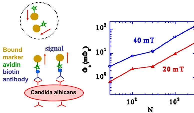
**Fig. 2.** Enpuku et al. Fig.9: Left – schematics of fungus detection method. Right: Detected signal versus the number of detected fCandida albicans fungi.
