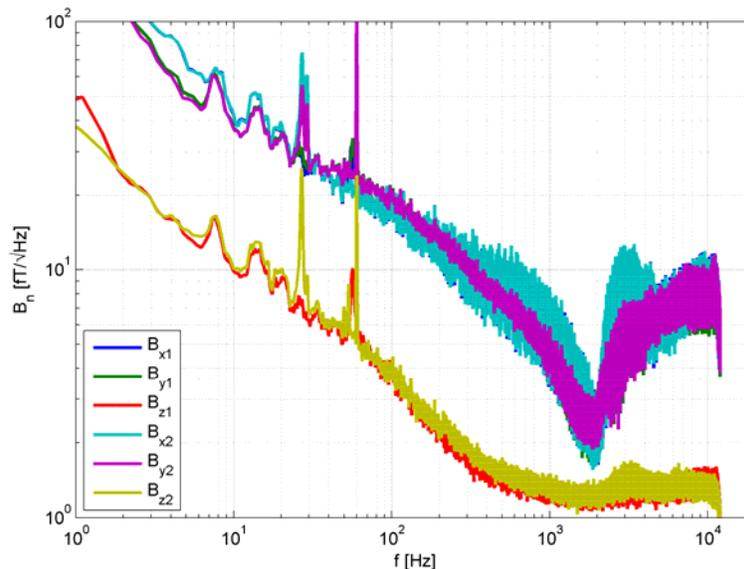
**Figure 1: Unshielded noise of 2 high sensitive SQUID triples, acquired simultaneously NW of Delta, Utah, USA. Note the good correlation between the channels in parallel, obviously we mostly see external signal.**
