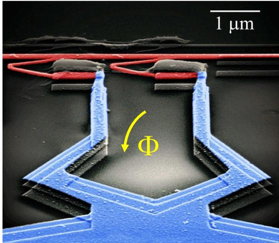
**Fig. 1:** Pseudo-color scanning electron micrograph of the heat interferometer. The hot (red) branch is heated up to  $\sim 500$  mK through a tunnel-connected source electrode whereas the cold (blue) branch is kept at the bath temperature  $\sim 250$  mK. Under these circumstances, the temperature of a drain electrode tunnel-connected to the hot SQUID branch was measured as a function of the magnetic flux  $\Phi$  threading the loop.
