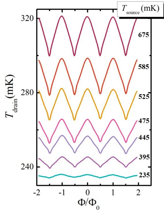
**Fig. 2:** Temperature modulation of the drain electrode  $T_{\text{drain}}$  vs.  $\Phi$  for different values of the temperature of the source electrode  $T_{\text{source}}$ . As predicted by the theory,  $T_{\text{drain}}$  is  $\Phi_0$ -periodic in  $\Phi$ , like the Josephson critical current.
