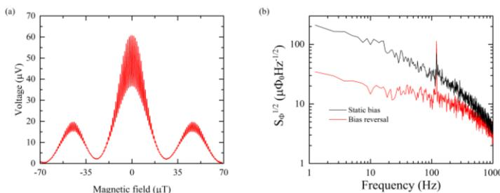
**Fig. 2.** Data for a SNS DC washer SQUID measured at 50 K adapted from [3] (a) Voltage as a function of magnetic field for static bias. Both the interference and diffraction pattern are visible; (b) Noise spectrum measured in a flux locked loop using both static and ac bias. © AIP 2015
