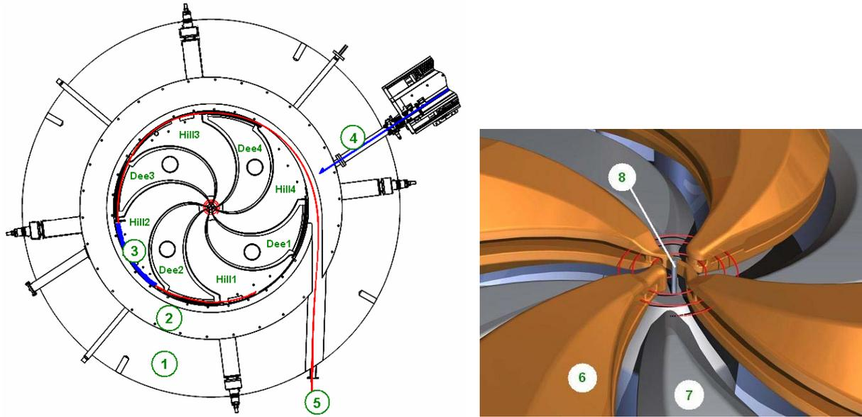
**Fig. 2.** Simplified median plane cut and central region 3d model of the cyclotron showing the main components. First spiral orbits of the proton beam in the central region and the beam extraction process are indicated in red.
