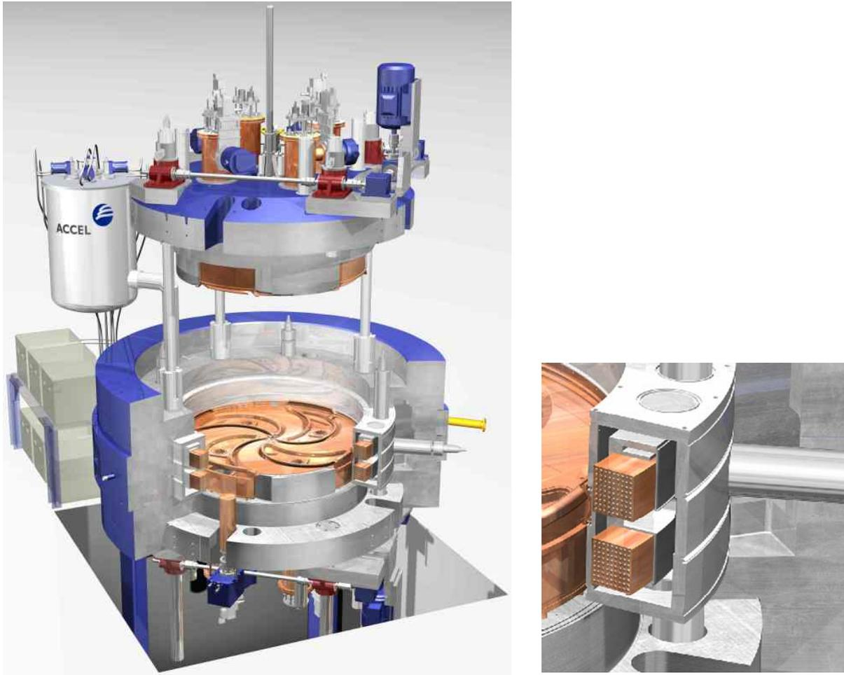
**Fig. 1.** Model cut view of the cyclotron with lifted upper pole cap (left) and detail showing the superconducting coil in the cryostat (right).
