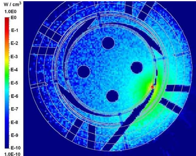
**Fig. 3.** Power density of neutrons produced by a 250 MeV proton beam that is stopped inside the cyclotron; color coded logarithmic scale ranges from  $10^{-10}$  to  $10^0$  W/cm<sup>3</sup>.
