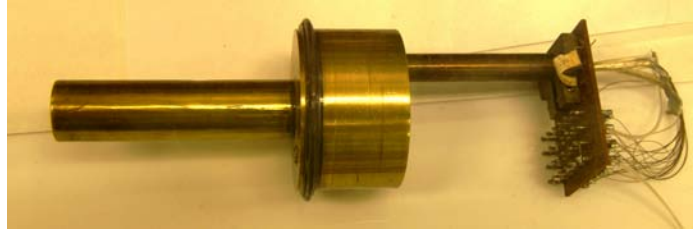
Fig. 4. Ian K. Harvey's superconducting current comparator [11].
