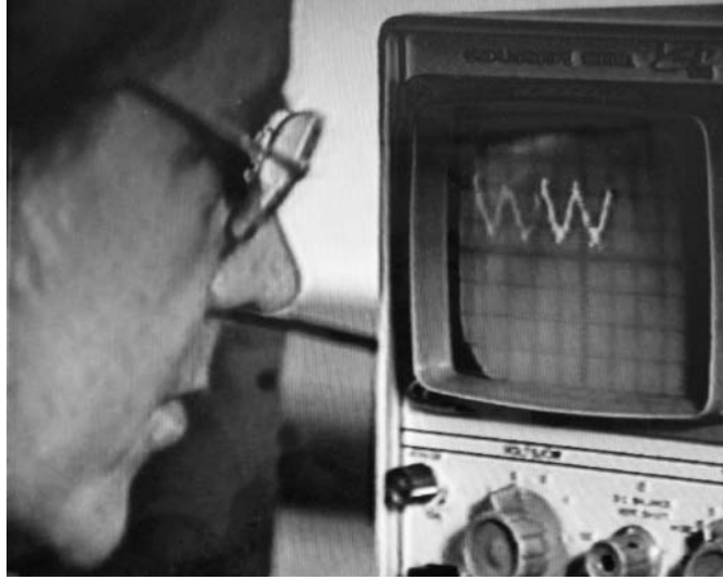
Fig. 5. Ian Harvey observes the triangular voltage vs. flux trace of an rf SQUID.
