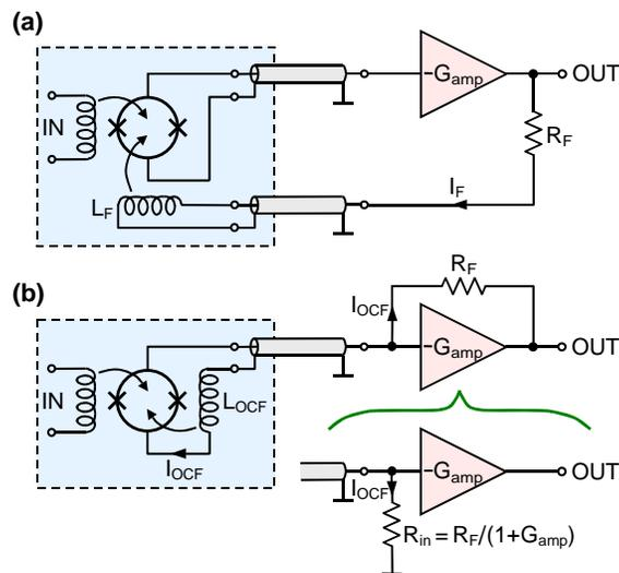
**Fig. 6.** Comparison of (a) the standard direct-coupled FLL and (b) SQUID linearization by OCF [29]. The whole SQUID circuit is represented by the usual single device symbol, with bias circuit omitted for clarity. The light blue area is at cryogenic temperature. The right lower corner shows the simplified equivalent circuit of the room-temperature SiGe amplifier.
