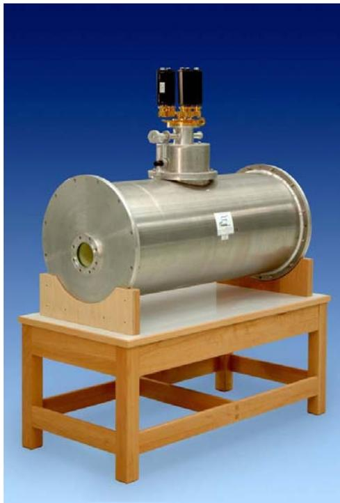
**Fig. 3.** Small animal scanner with horizontal warm bore.
