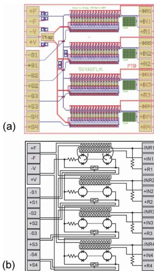
**Fig. 2.** Layout (a) and basic circuit diagram (b) of the integrated time division SQUID multiplexer chip C5X416FLM. The chip size is  $3 \times 3 \text{ mm}^2$ . Circuit details are omitted for clarity.
