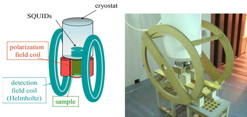
**Fig. 4.** Low-field NMR setup. Left: sketch of single-channel SQUID detection of low-field Larmor precession. The polarization field generated magnetization along the y axis. After switching off the polarization field, sample magnetization begins to precess about the z axis of the detection field. Right: Photo of the LF-NMR setup operated in BMSR-2.
