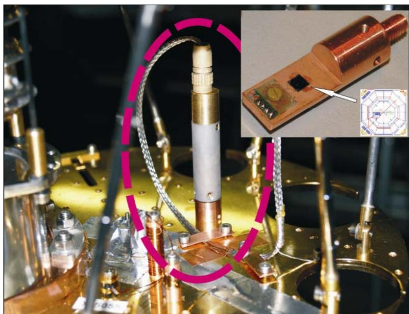
**Fig. 5.** The magnetic field fluctuation thermometer (MFFT) mounted on the mixing chamber plate of a  $^3\text{He}/^4\text{He}$  dilution refrigerator. The insert shows the open MFFT with Cu block and the mounted radial SQUID gradiometer chip  $3 \times 3 \text{ mm}^2$ .
