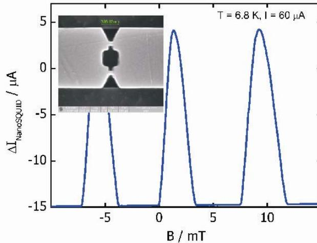
**Fig. 1.** Current-flux characteristics of a nanoSQUID (NPL) read out with a 16 SQUID series array current sensor (PTB). The inset shows the SEM image of the nanoSQUID with nearly square loop size of  $370 \times 370 \text{ nm}^2$ .
