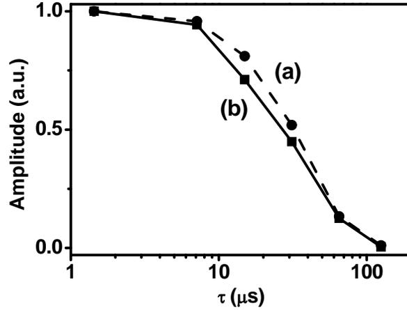
**Fig. 3.** Theoretical (a) and experimental (b) normalized initial amplitude of FID signals *versus* the decay time constant;  $f_L = 4.23$  kHz.
