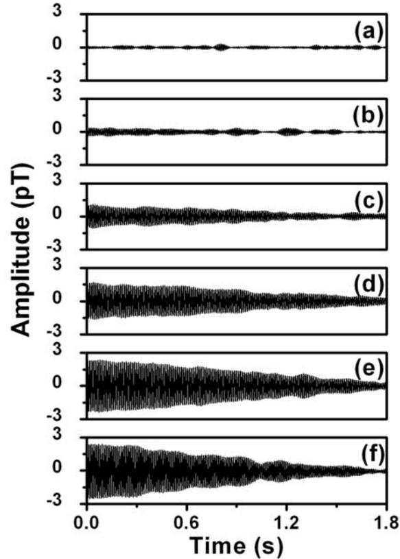
**Fig. 2.** FID signals of 10 ml tap water with different shunt resistors;  $f_L = 4.23$  kHz. Traces (a) to (f) correspond to shunt resistance  $R$  of 47 $\Omega$ , 100 $\Omega$ , 220  $\Omega$ , 470  $\Omega$ , 1000  $\Omega$ , and 5000  $\Omega$ , respectively. (signals averaged,  $N = 10$ )
