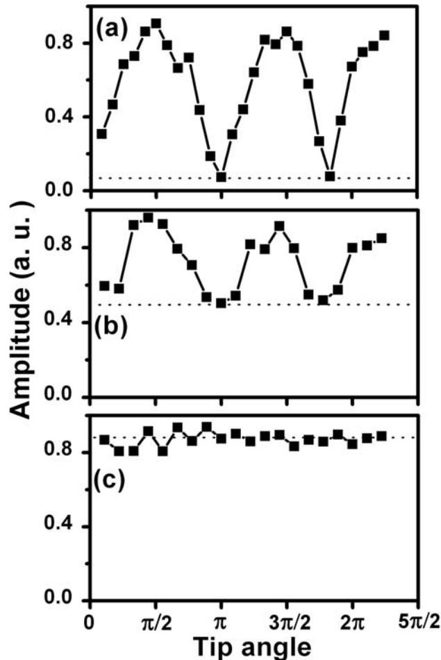
**Fig. 4.** Signal recovering with an *ac* pulse when  $f_L = 4.23$  kHz,  $B_p \perp B_m$ . The shunt resistance in curves (a) to (c) is  $R = 47 \Omega$ ,  $470 \Omega$  and  $5000 \Omega$ , respectively; they illustrate the situations of the NMR signal totally destroyed, partly destroyed and hardly affected. The dotted line in each figure shows the signal level without the *ac* pulse.
