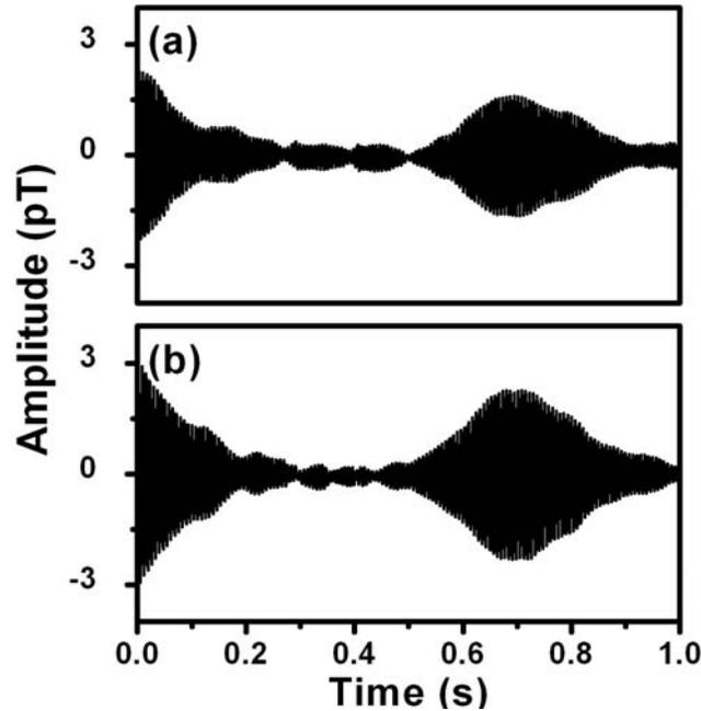
**Fig. 5.** FID and a spin-echo signal with  $B_p \perp B_m$  (a) and  $B_p // B_m$  (b). The  $\pi/2$  and  $\pi$  pulse are applied 5 ms and 350 ms after switch-off of  $B_p$ . In both cases, the shunt resistance is  $47 \Omega$ , and after averaging ( $N = 50$ ).
