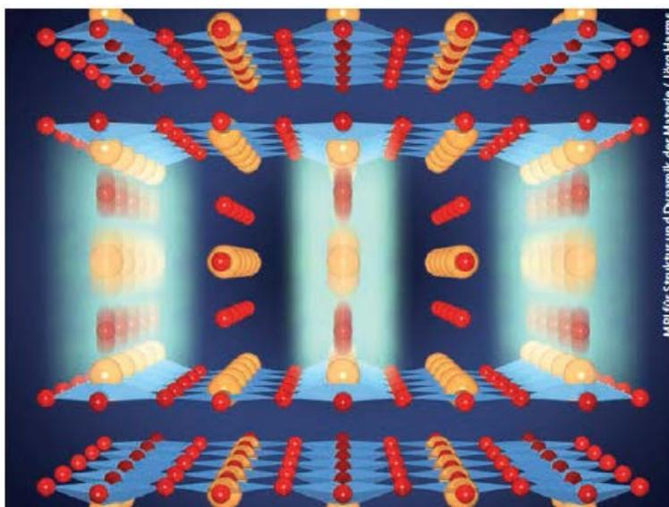
**Fig. 1.** Structure of  $\text{YBa}_2\text{Cu}_3\text{O}_{6+\delta}$   $\text{CuO}_2$  double layer (light blue),  $\text{CuO}_3$  chains perpendicular to the projection plane, Cu atoms (orange), O atoms (red). Due to resonant excitation of apex O atoms (blurred), which are in between the double layer and the chains, the atoms are moved out of their equilibrium position.
