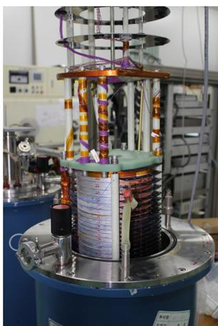
**Fig. 1** Assembled magnet and liquid He Dewar.
