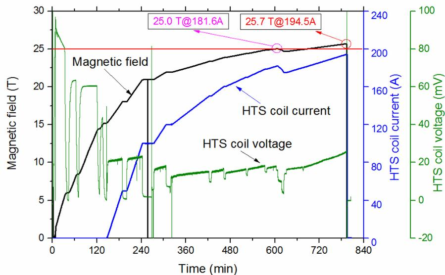
Fig.2. Test of the REBCO insert under 15 T background magnetic field at 4.2 K
