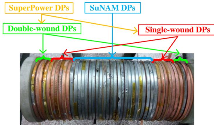
Fig.1. REBCO insert in assembly
