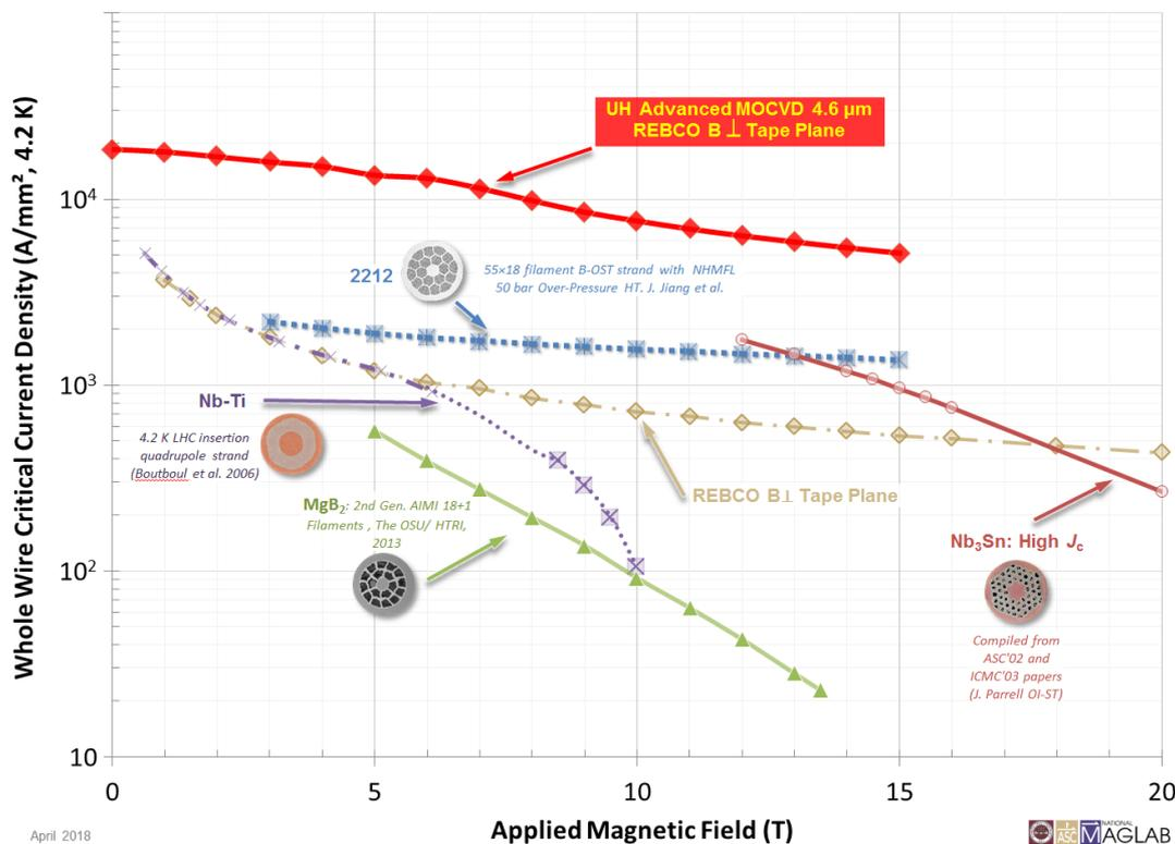
**Fig. 1.** Engineering current density vs. field of thick UH REBCO tape and other technical superconductors at 4.2 K [3].
