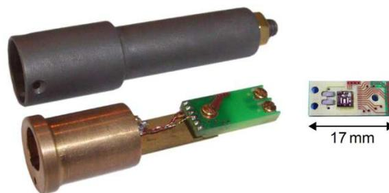
**Fig. 12.** Example of a commercial SQUID package. The superconducting connection to the input coil is realized via screw contacts. For low-noise operation, the SQUID carrier is enclosed by a Nb shield. On the left side, the socket for the wiring to the room temperature electronics is visible (courtesy of Magnicon GmbH, Hamburg).
