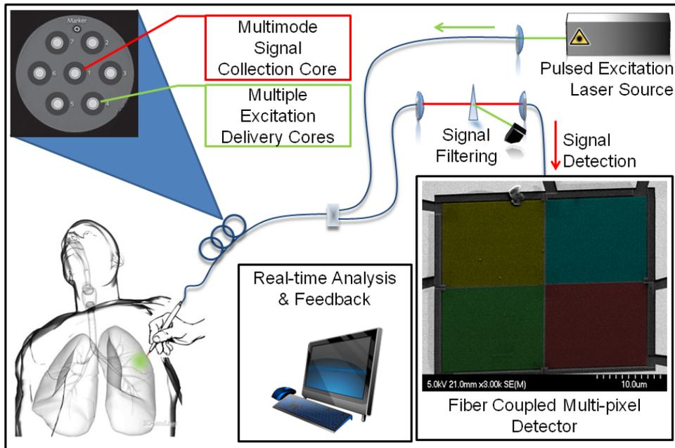
Fig. 3. An example of the future application of the system described. A Multiple core fiber delivery and collection system allows the detector to be housed remotely from the operating theatre. Next generation multiple pixel detector systems will allow the coupling of multimode fiber vastly increasing collection efficiencies and allowing real-time feedback to clinicians.
