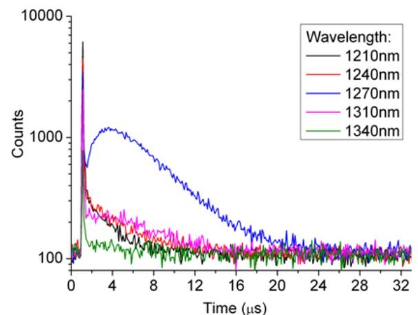
Fig. 1. Representative TCSPC histograms with a SNSPD from Rose Bengal photosensitizer solution (250 μg/ml, 0.257 μM) with bandpass filters (20 nm spectral width) centred at 1210, 1240, 1270, 1310 and 1340 nm [10 min acquisition time, 0.1024 μs bin size]. Short-lived fluorescence (occurring within the first μs) is present at all wavelengths studied; the key signature of <sup>1</sup>O<sub>2</sub> is the onset and decay that is observed only at 1270 nm.
