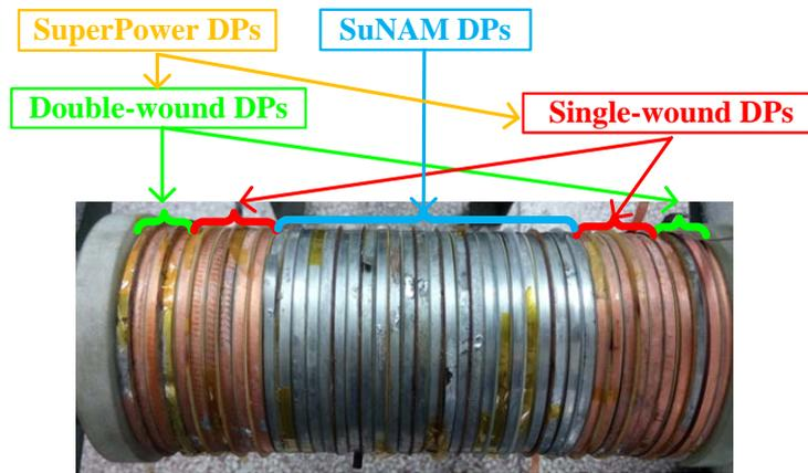
Fig.1. REBCO insert in assembly
