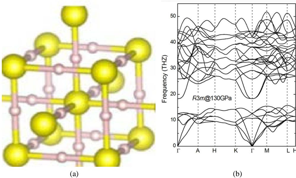
**Fig. 1.** (a) The high- $T_c$  ( $\approx 200$  K) phase is cubic [5]. (b) Phonon spectrum for the high- $T_c$  ( $\approx 200$  K) phase. It contains two groups: (1) acoustic modes (up to  $\sim 70$  meV, motion of the S ions) and (2) optical modes (up to  $\sim 200$  meV, dominated by the motion of the H ions).
