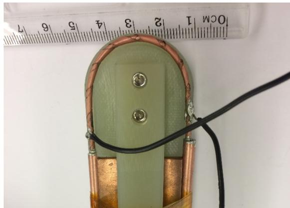
**Fig. 2.** REBCO STAR wire mounted for critical current testing on a G-10 fixture, bent at 15 mm radius along with its copper terminals
