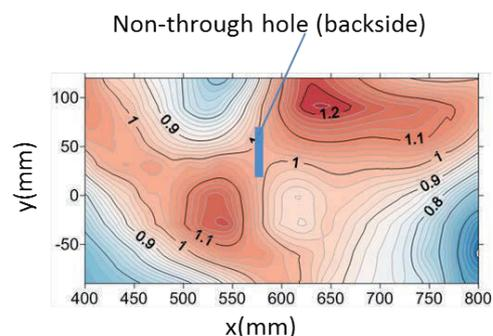
**Fig. 1.** Magnetic field pattern (real part) of a 6 mm thick steel plate with a backside defect.
