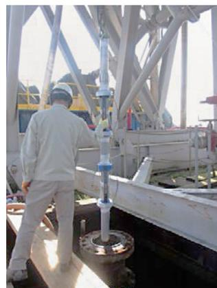
**Fig. 2.** SQUID receiver system put into a well at JOGMEC Kashiwazaki test field.
