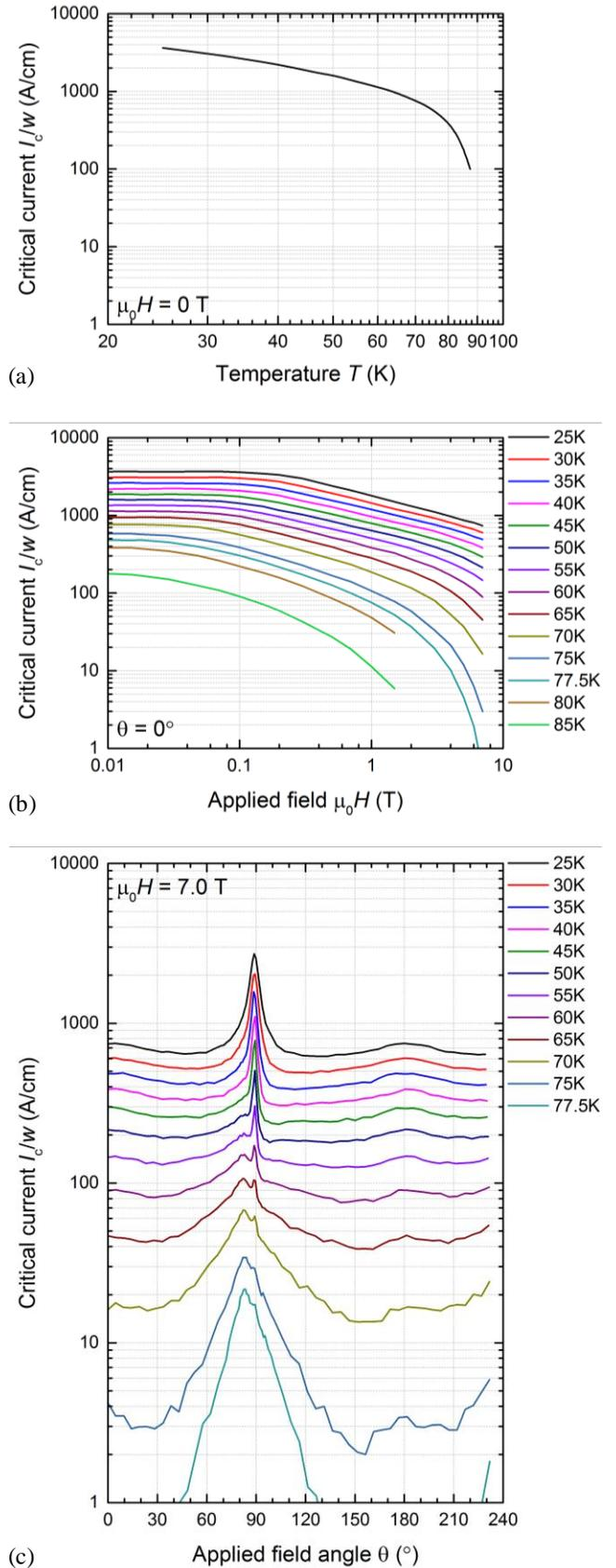
Fig. 1. Graphs showing the (a) temperature, (b) field, and (c) angle dependence of the critical current of an STI Conductus<sup>®</sup> wire sample under the specific conditions noted on the graphs, as an example of the standard measurement types included in a dataset.
