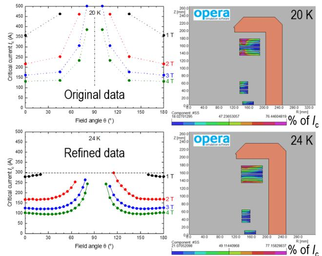
Fig. 3. Results of modelling the  $I_c$  utilization of a 1.5 T HTSMRI coil using an original and refined wire characterization dataset. A similar maximum  $I_c$  utilization of 77% is obtained at an operating temperature of 24 K after refinement as was obtained at 20 K using the original data.
