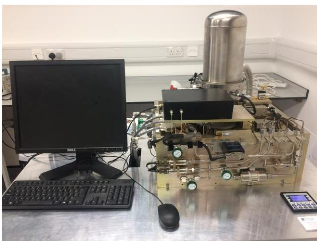
**Figure 2** Miniaturized 4 K cooler for SNSPDs developed in partnership with STFC Rutherford Appleton Laboratory.
