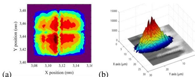
**Figure 1** SNSPD development at Glasgow (a) photoresponse map of  $60\ \mu\text{m} \times 60\ \mu\text{m}$  area four-pixel SNSPD array with peak detection efficiency  $>40\%$ . (b) waveguide integrated SNSPD [3].
