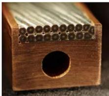
Fig. 2. Picture of the cross-section of the Rutherford cable on conduit conductor (RCOCC) produced. The dimensions are given in Table I.
