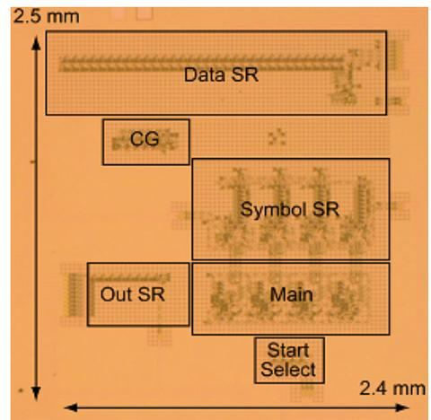
Fig. 3. Microphotograph of an 8-bit 4-symbol SFQ CED circuit with an on-chip high-speed test system.
