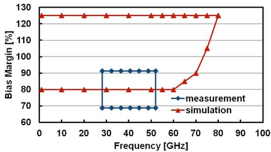
Fig. 6. Simulated and measured bias margins of the 8-bit 4-symbol SFQ CED circuit as a function of clock frequency
