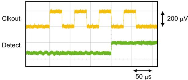
Fig. 5. Output signals of the “Pattern 2” in the measurement. Each transition in the waveforms corresponds to the output of an SFQ pulse.
