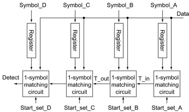
Fig. 1. A block diagram of a 4-symbol SFQ CED circuit
