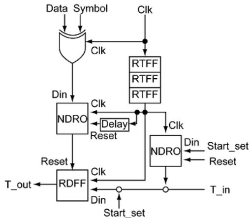
Fig. 2. A circuit diagram of the SFQ 1-symbol matching circuit
