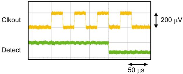
Fig. 4. Output signals for the “Pattern 1” in the measurement. Each transition in the waveforms corresponds to the output of an SFQ pulse.
