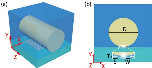
Fig. 1. (a) Schematic diagram of the microfiber-integrated SNSPD. (b) Cross section of the structure. Inset indicates the interface between microfiber and NbN nanowires.
