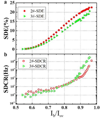
Fig. 2. SDE (a) and SDCR (b) as functions of the normalized bias current ( $I_b/I_{sw}$ ) for two microfiber-coupled SNSPD
