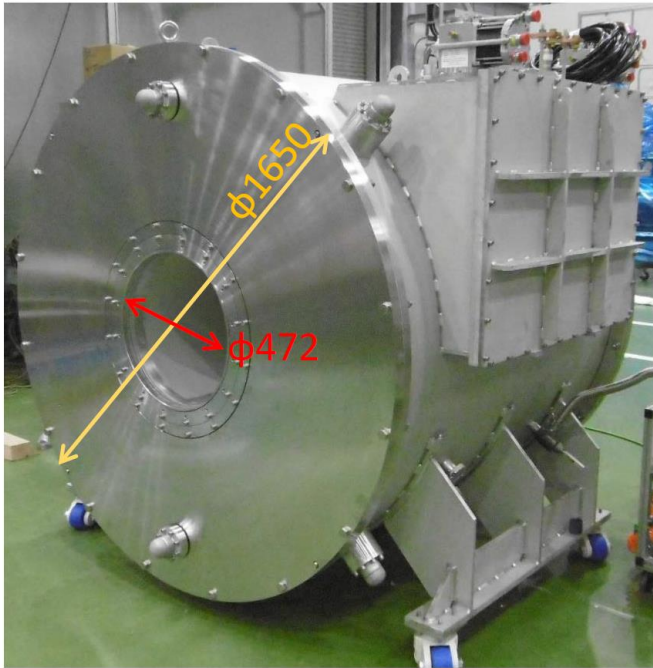
Photograph of a Cryostat (Max : W1881-Z1672-H1790)
