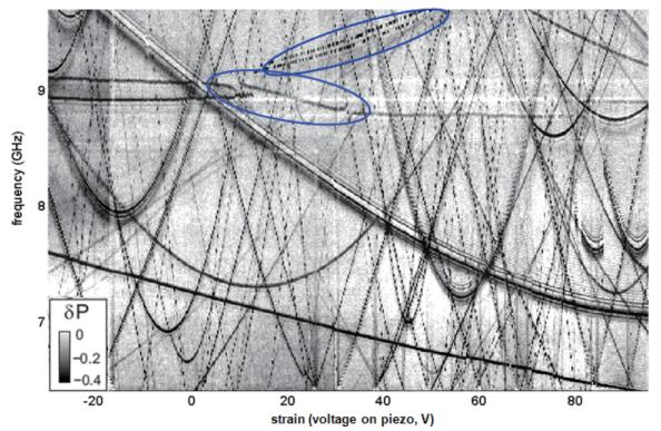
Figure 1: TLS spectroscopy, showing the resonance frequencies of strain-tuned individual TLS as dark traces. Encircled are anomalies which provide evidence of mutual coupling between TLS.
