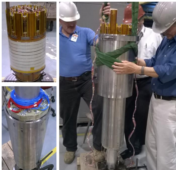
Fig. 10. Outer coil with 16 pancakes (top-left), inner (bottom-left) coil with SS support tube and outer coil with support SS support tube being installed over inner tube (right).
