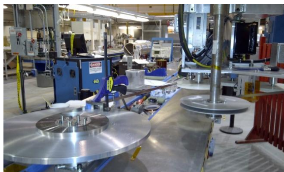
Fig. 6. Computer-controlled universal coil winding machine used for winding inner and outer pancake coils.
