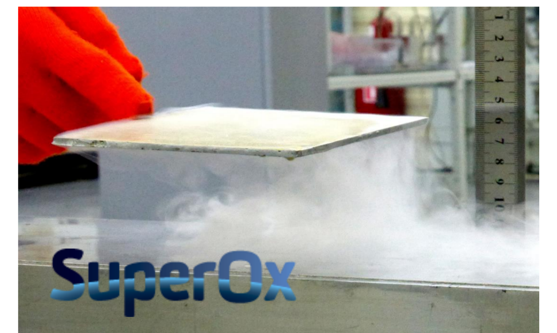
By overlapping standard 12mm wide HTS commercial tape, composite bulk slabs can be fabricated with potentially unlimited size.
