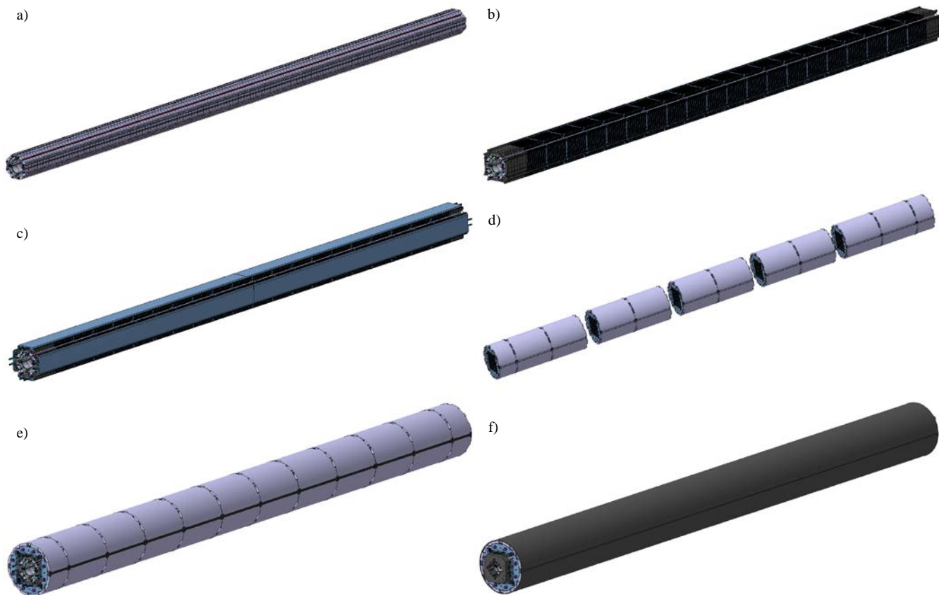
Fig. 7. Components of the MQXFB cold mass: collars (a), pads (b), masters (c), yoke and shells (d,e), LHe vessel and axial loading system (f).
