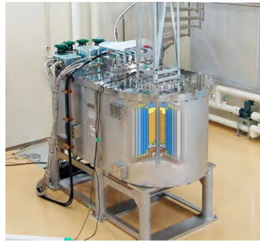
Fig. 2. Photo of the 25T-CSM installed at the HFSLM annex building.
