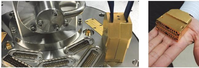
Fig. 5. Compact 20-channel interface amplifier unit was developed to connect directly to a 20-G3PO coaxial vacuum feedthrough. A pair of twinax cables carry the differential outputs from the two 10-channel circuit boards to the FPGA data receivers.
