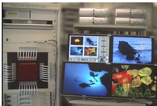
Fig. 4 Demonstration of video transfer between four PCs through an SFQ 4x4 switch.
