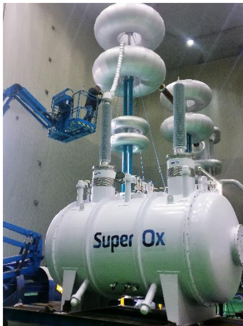
Fig. 5 220 kV SFCL phase at the KERI test center.
