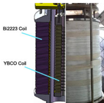
Fig. 1. Configuration of assembled insert coils.
