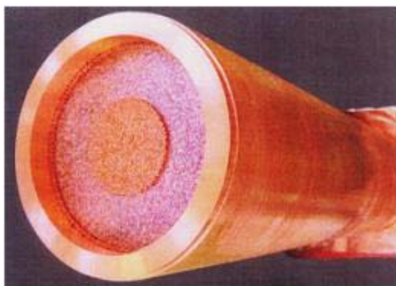
Fig.2. An assembled Nb-Ti billet for extrusion. Outer diam.: 236.5mm, Number of Nb-Ti cores: 8500, Center: Cu rods [4].
