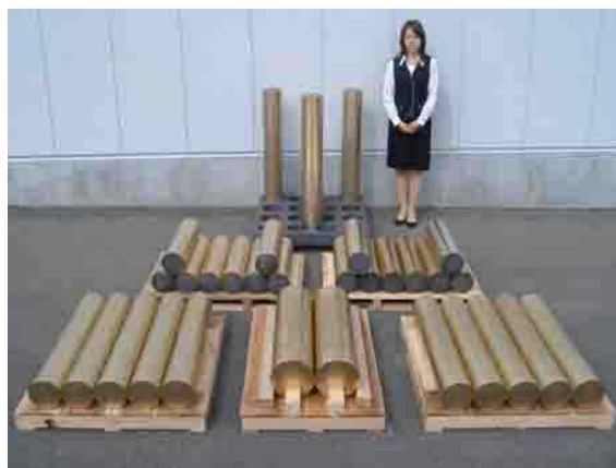
Fig.10. Typical bronze ingots for Nb_3Sn wires (Courtesy of Osaka Alloying Works Co., Ltd.) [19].
