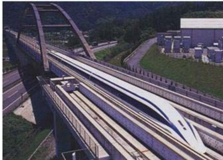
Fig.4. In 2008, the superconducting magnetically levitated train reached the speed of 581km/h [5].
