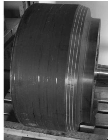
Fig. 3. Multirim flywheel rotor.
