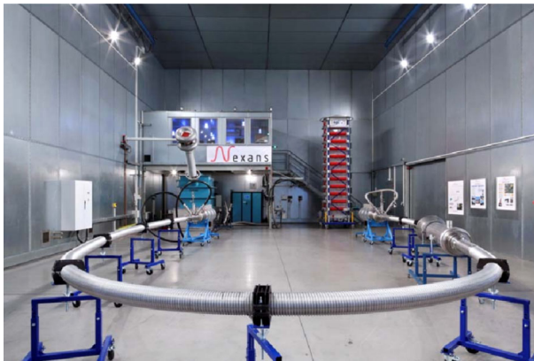
Fig. 21 Prototype of the AmpaCity cable and accessories setup for type test in laboratory [153]
