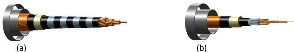
Figure 1. Typical superconductor cables' layouts. a) Multilayer HTS cable; b) Multistage MgB 2 cable.
