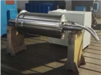
Superconducting rotor system
