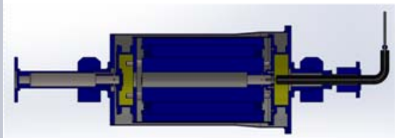
Cryogenic system of the HTS generator
