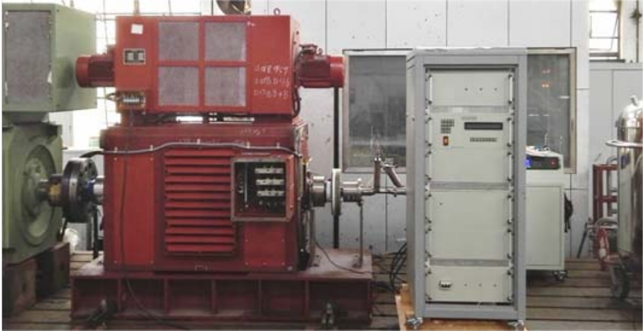
500 kW HTS generator system
