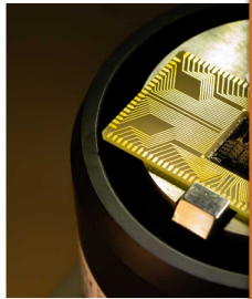
Photo: Christopher Ayala The AQFP-based MANA microprocessor die contains over 20,000 superconductor adiabatic superconducting microprocessors.
