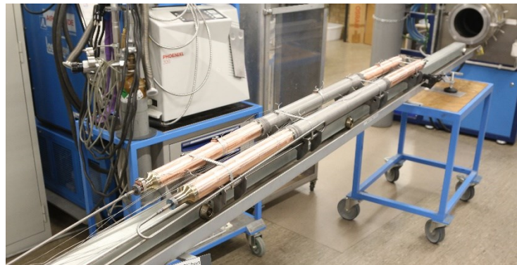
4 conductor sections heat treated at PSI
