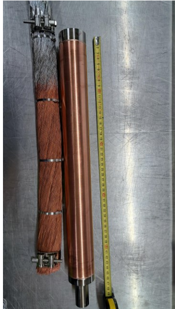
4 conductor sections heat treated at PSI
