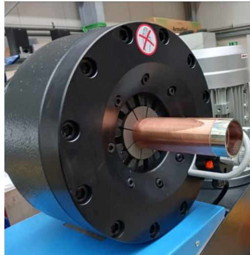
Crome etching and crimping of the Cu tube on the CiCC
