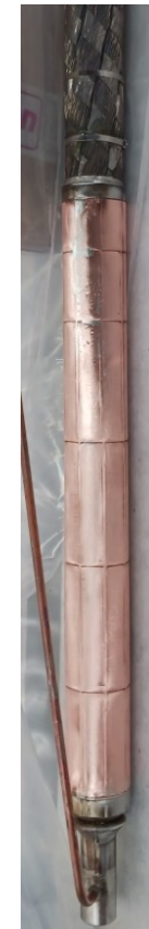
Scarf joint 15-degree pre-cut
