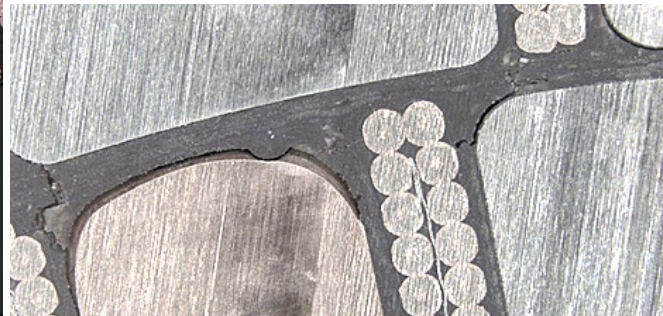
Cracking and resin adhesion issues (metallic components, strands)
