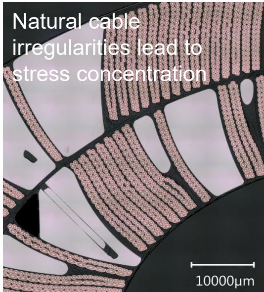
Cracking and resin adhesion issues (metallic components, strands)
