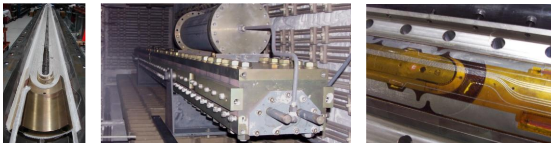
FIGURE 6. LQ coil after winding (left), in the reaction tooling (center), and after impregnation (right).
