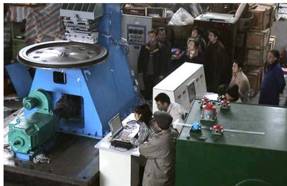
Fig. 21. HTS Maglev dynamic test system (SCML-03)
