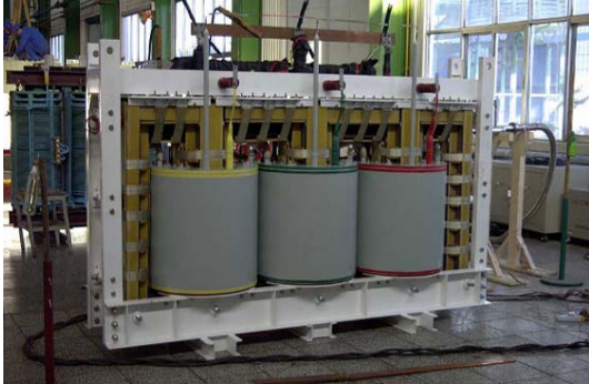
Fig. 17. Overview of the 630 kVA 10.5 kV/0.4 kV transformer
