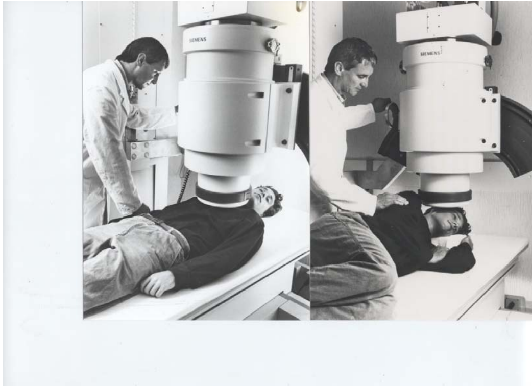
Fig. 5. The “Krenikon” 37-channel biomagnetometer used to measure human subject’s heart and brain magnetic field activity (courtesy of H.E. Hoenig and Siemens AG – Sector Healthcare, “MedArchiv”).
