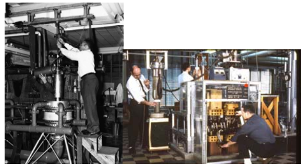
Fig. 1. (Left) Dr. Warren Henry performing research at cryogenic temperatures in NRL's high magnetic field facility demagnetization (Right) Dr. Robert Hein using adiabatic demagnetization to test the properties of superconducting materials at temperatures to 10 mK.
