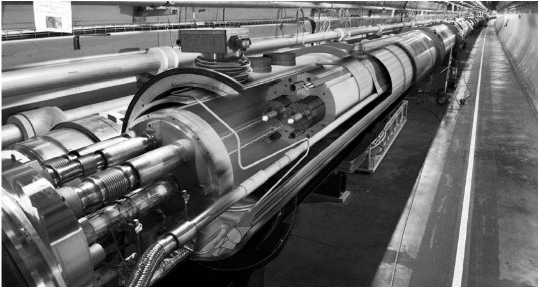
FIGURE 13. The LHC tunnel, with cutaway representation of a dipole magnet in the foreground (photo CERN).
